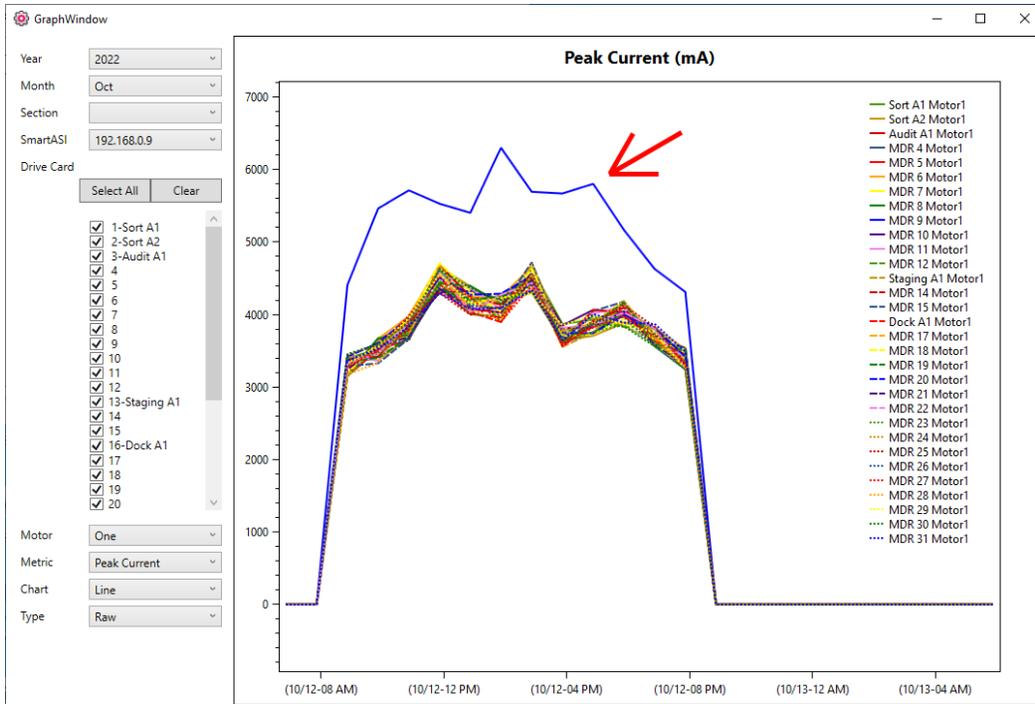
This example is charting peak current using a line graph. Clearly there is a huge outlier in the data as signified by the red arrow. This motor will likely need to be replaced soon.
