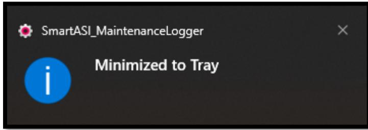
When the MaintenanceLogger is first started or when it is minimized, the above notification will be displayed and the window will be minimized to the system tray. You can open the MaintenanceLogger by either clicking this notification, or double or right clicking the Icon in the system Tray:
