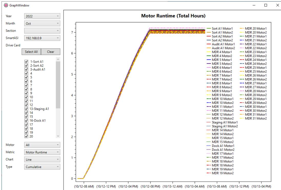
In this example the cumulative runtime of the motors has been graphed. This data can be used to track how close a motor is getting to its expected life expectancy. Additionally in this example both motors are being graphed for each drive card.
