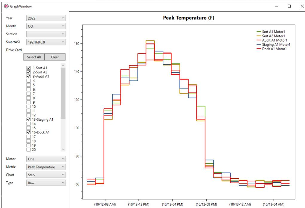
In the above example, Conveyor sections have been created for several Drive Cards, giving them descriptive names in both the Drive Card list and in the legend of the graph. A step graph is being used, giving a more accurate view of when the data was collected. Only a few Drive cards have been enabled in this example.
