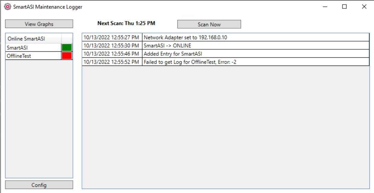
The SmartASI Maintenance Logger is an accompanying software for the SmartASI PLC/Gateway. It starts up automatically with the PC and proceeds to log maintenance data from the SmartASI at a user-defined interval. The data can then be filtered and viewed in a graph window. Additionally, a message log will be kept and will show whenever an error or anomaly occurs on the network, such as a SmartASI going offline.
