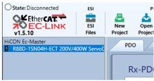
Once a slave is selected, you should see a number of PDO mappings appear in the Rx and Tx PDO sections. Here you can choose which PDOs to use by clicking the checkbox next to the PDO.
