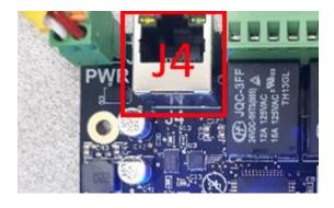
Connect another Ethernet cable from the router to your PC. The router will dynamically assign a unique IP address to both the PC and the HiCON. This completes the network setup without requiring any intervention from the user.
