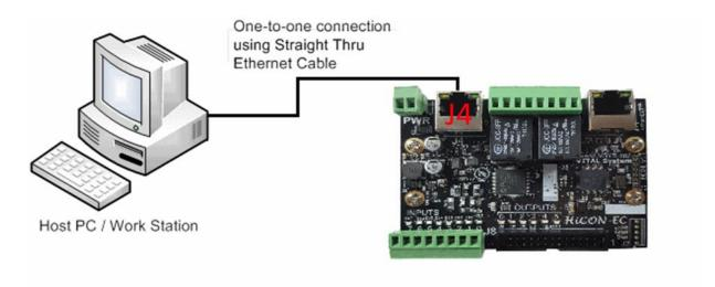
When this configuration is used, the network address of the EC01 must match that of the PC's ethernet adapter. The default IP address of the HiCON board is 192.168.0.95. This means that we must change the PC's adapter IP to a static IP with the form 192.168.0.xxx. The following steps will demonstrate how to accomplish this.
