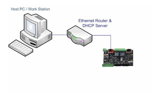
This is the simplest method to connect Mach software to the controller. The figure above shows a basic setup using an Internet router on your network. Connect the Ethernet cable from the J4 Ethernet port of the HiCON to the router.
