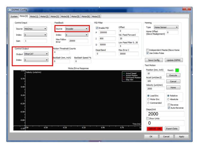
The marked entries indicate the EtherCAT-specific configuration.
