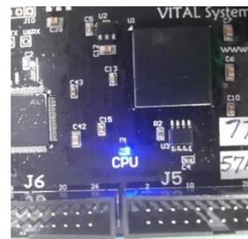
3. If the DSPMC is correctly powered up as seen above, the green power LED should be lit and the blue CPU LED blinks in some pattern.
