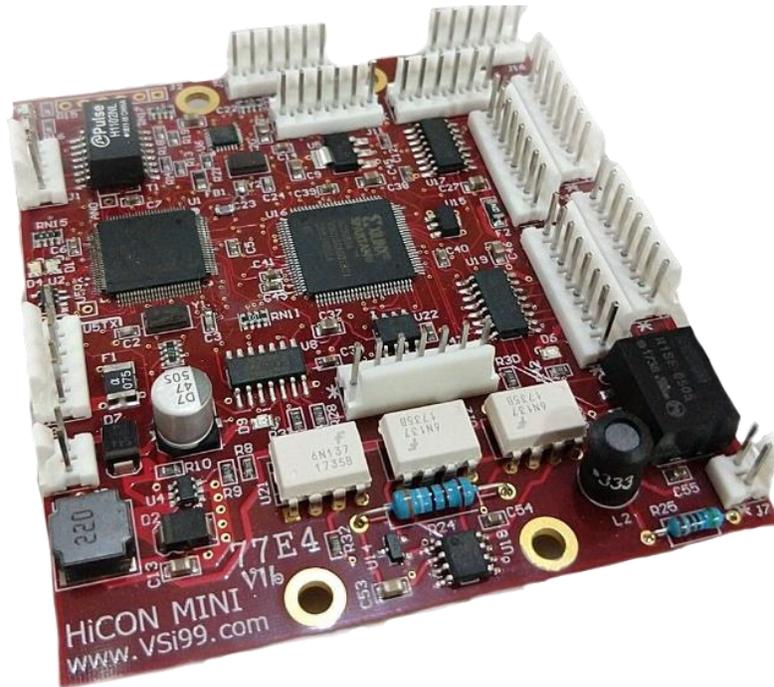
The HiCON Mini is an Ethernet based controller for motion control, data acquisition, and general PID control system applications. Utilizing the latest Microchip technology, the HiCON Mini offers a comprehensive set of features for your demanding applications.
