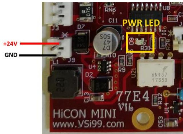
3. If the HiCON Mini is correctly powered up, the 24V LED at D9 should be lit up to indicate that the voltage is present on the unit, and the CPU LED at D4 should blink in a constant time.
