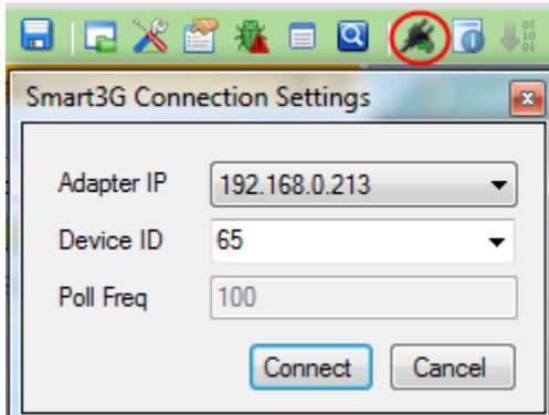
Although SuperLogic Pro can compile Ladder-Logic programs, running them requires a connection to a Smart3G Device.
