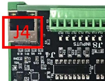
Connect another Ethernet cable from the router to your PC. The router will dynamically assign a unique IP address to both the PC and the HiCON. This completes the network setup without requiring any intervention from the user.
